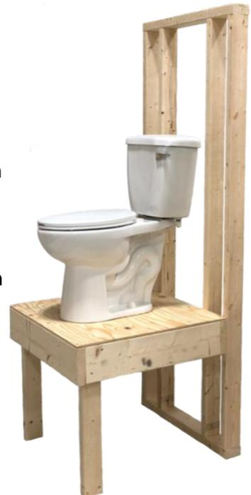
Each unit can be utilized with PVC, CPVC, PEX, and Copper. The elevated floor allows for the systems to be connected together to experiment with multi-fixture systems, water supply and DWV connections.
